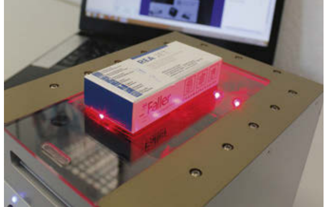
DataMatrix code verification on product packaging
