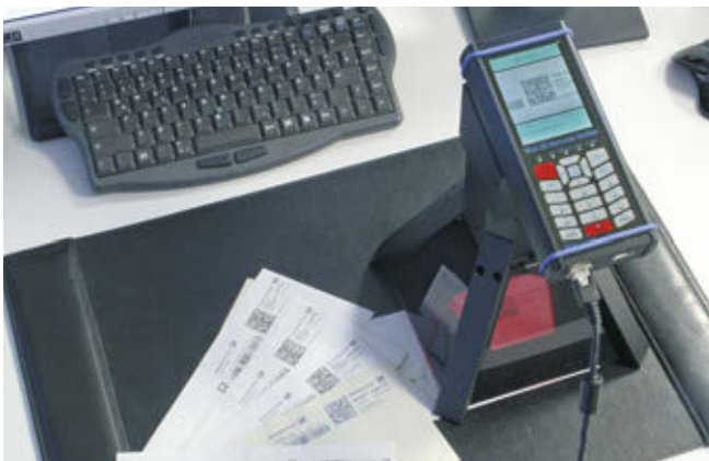
Verifying DataMatrix codes on mailing bags
