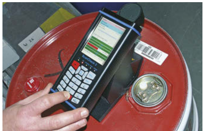
Verifying barcodes on metal barrels
